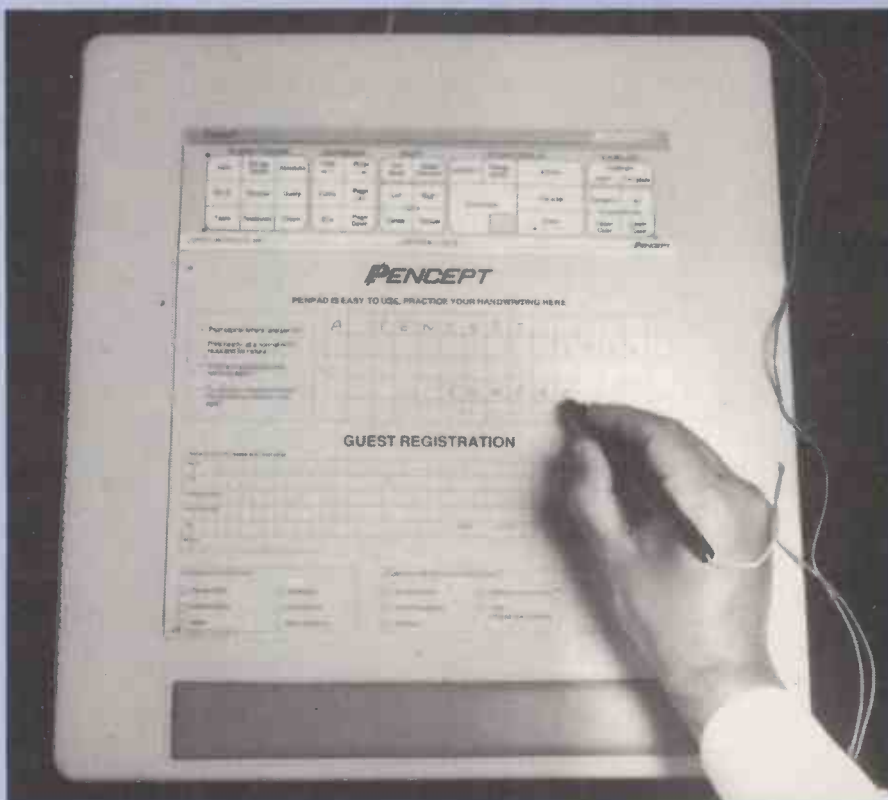
The Penpad accepts inputs from a magnetic stylus. A microswitch in the head detects when it is in contact with the pad's surface, and a small button on the side allows it to be used in a mouse-like way.
